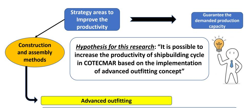
Strategy currently used by the most modern shipyards in the world and allows the installation of the largest amount of equipment (machinery, pipelines, cables, etc.) in the earliest stages of construction, especially during pre-assembly and assembly of each block that compose the hull.
